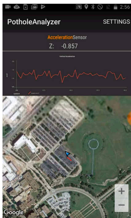
Figure 2. The user interface of PotholeAnalyzer .
