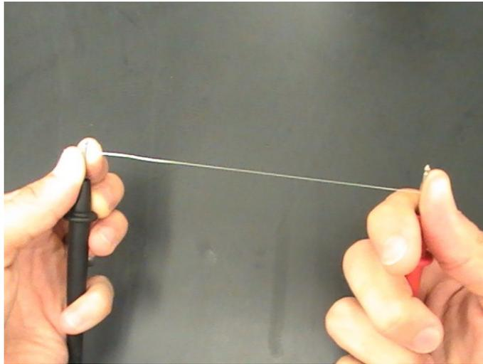
**Figure 2.** Checking for breaks in Teflon-coated wire using a multimeter (FLUKE 73II). One exposed end (approximately 0.5 cm) of the wire was then inserted into the tip of a needle (26G<sup>3/8</sup>, Intradermal Bevel) and the remaining length of the wire was coiled 7-8 times around the needle (see *Fig. 3*).
