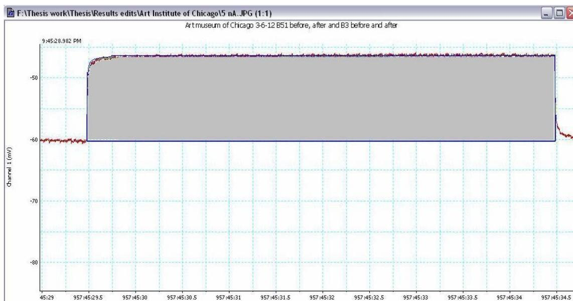
**Figure 11.** The grey square above represents the area underlying the  $K^+$ -dependent depolarization. All of the points comprising the area were selected (blue outline above) and the ImageTool® software calculated the area.
