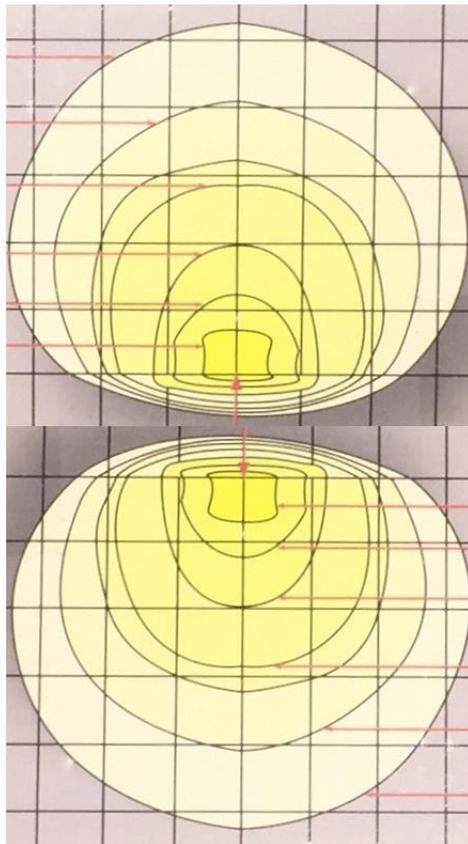
*Figure 1. Spatial light distribution pattern produced by the two floodlight fixtures equipped each with a 400-watt metal halide lamp used as light source for bioreactors according to specifications provided by the manufacturer.*
