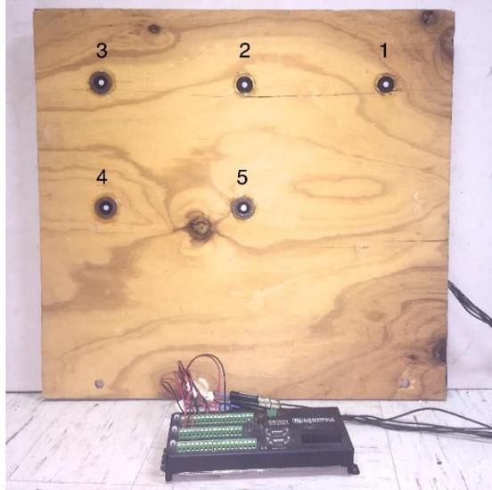
Figure 2. Five-quantum sensor outfit used to collect incident and transmitted photosynthetic photon flux density data on the lit and unlit sides of bioreactors.
