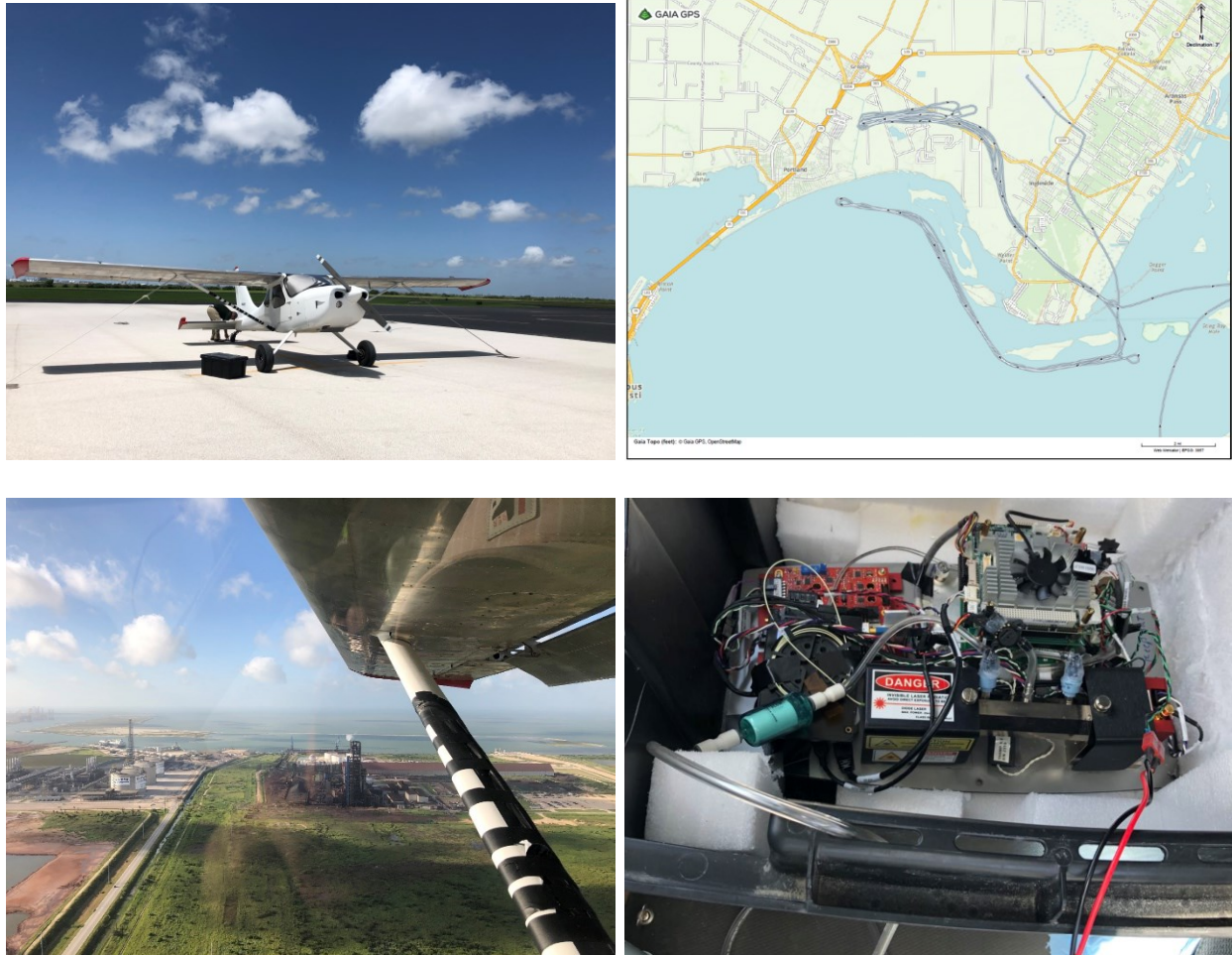
Figure 5.3 Upper Left: aircraft applied in this study; Upper Right: flight routes; Lower Left: Smoke from a tower (Voestalpine Texas) at the Ingleside industrial area during the flight; tubing was tied under the wing to collect air samples; Lower Right: the assemblies of gas inlet, gas measurement, system control, and data storage of the Microportable Greenhouse Gas Analyzer.
