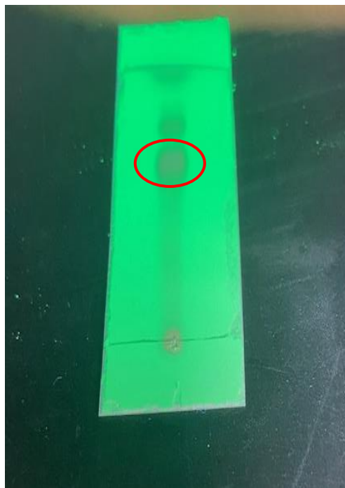
Figure 11. TLC result of the crude product of the ligand. The spot of the pure ligand was the spot circled in red. Individual fractions collected from first trial of column chromatography were examined with NMR to confirm the ligand spot position.
