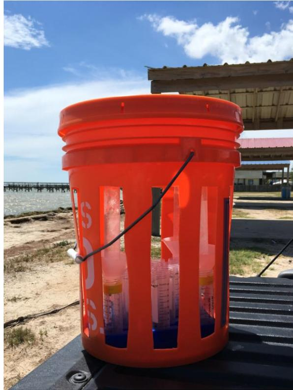
**Figure 13.** Photo of condensate collecting device with ice-filled test tubes and collection vials visible inside modified 5-gallon bucket.
