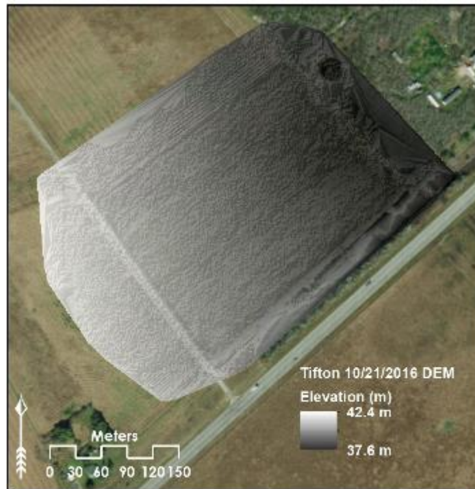
Figure 23. The UAS-SfM-derived digital elevation model for the October 2016 Tifton field flight.
