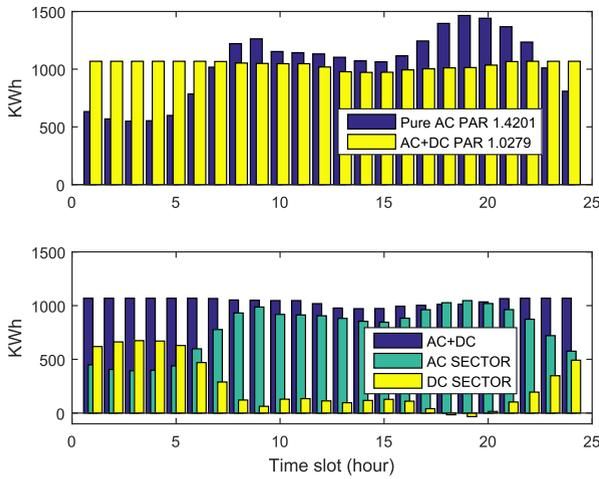
FIGURE 4. Distribution level and sector level scheduled load profiles.
