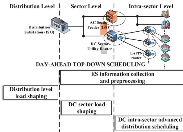
FIGURE 2. System topology and day-ahead top-down load scheduling.
