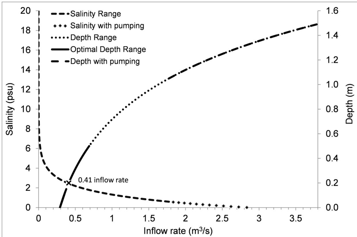
Figure 20: Relationship between Rincon Bayou pumping rates, salinity ranges, and depth ranges for the three indicator species at Station C.
