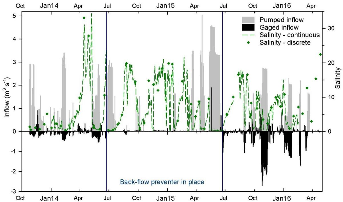
Figure 17: Pumped and Gaged inflow into Rincon Bayou and salinity at station C. Discrete salinity measurements were made simultaneously with fauna samples during the bi-weekly sampling period.
